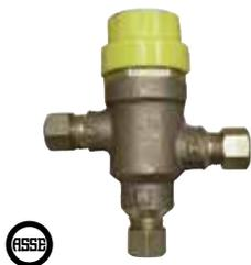
Apollo 34D Series thermostatic “Mini Mixer” valves are dual ASSE 1070 certified and designed as the ultimate single fixture valve, with a mixed accuracy of +/- 2° F. Two designs are available depending on the application; single outlet design for sensor type faucets and double outlet design for standard connections.
