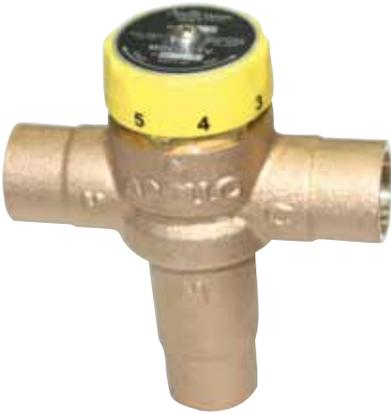
The Apollo® Model TV (34-200 Series) thermostatic mixing valve provides non-ASSE extension of water heater capacity and hot water temperature control in hydronic heating systems. Available in low or high temperature options for floor or baseboard applications.
