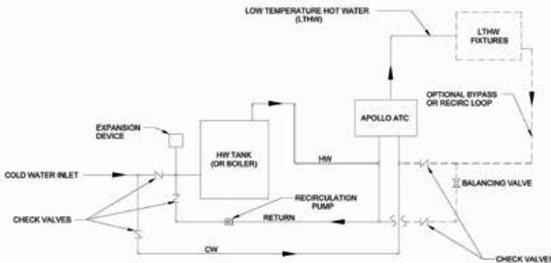
Figure 2: Typical Installation with Optional Recirculation loop
