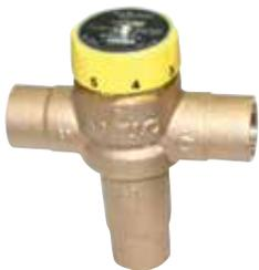
Apollo 34 Series mixing valves help extend hot water supply and enhance the life and accuracy of hydronic thermostats in residential and small commercial systems. These valves may be used to increase draw capacity of automatic storage water heaters. They save hot water and energy by automatically regulating the mix of hot water with cold. Water temperatures can be adjusted by simply turning the yellow knob to the desired setting.
